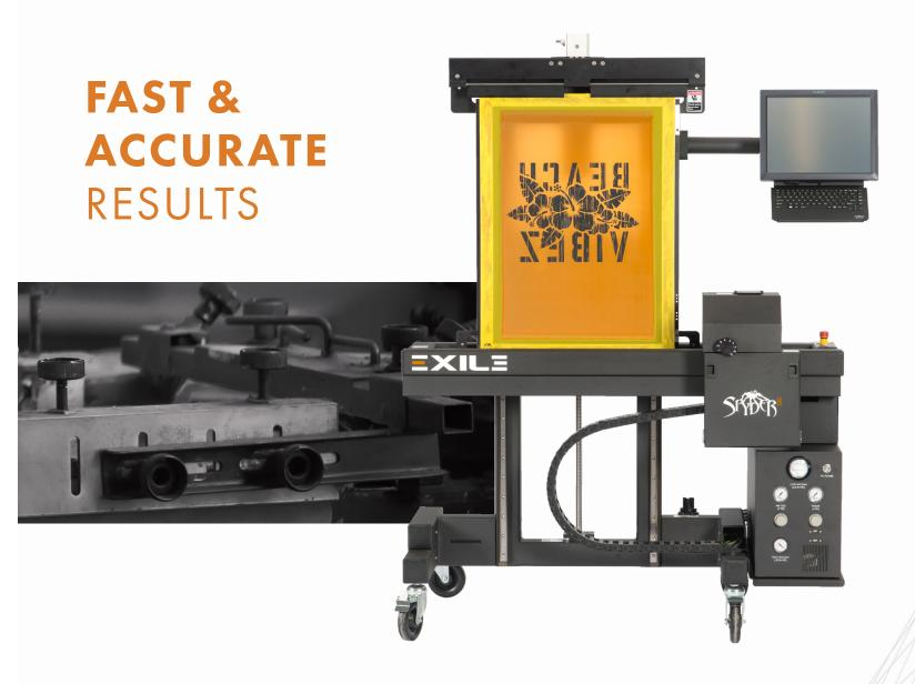
The Spyder II 30 supports standard frames up to 30"  $\times$  40", while the larger Spyder II 52 supports frame sizes up to 54"  $\times$  46". A full-featured Harlequin RIP is included to provide a fast and reliable file output. The Spyder II also accepts 1-bit tiff files from any other RIP to easily fit into an existing pre-press workflow.
