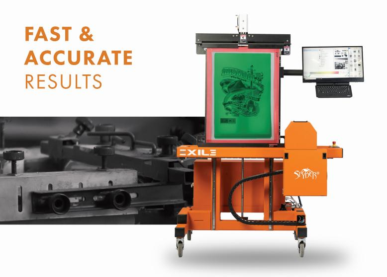
The Spyder III supports standard frames up to 30" x 40". The frames lock in precisely against a 3-point registration system which provides extremely accurate placement of the image from color-to-color, screen-to-screen. Once paired with the registration system on the printing press, multi-color jobs lock into place with very little, or no micro-registration. This results in extremely quick press setups and, ultimately, more jobs printed per day.
